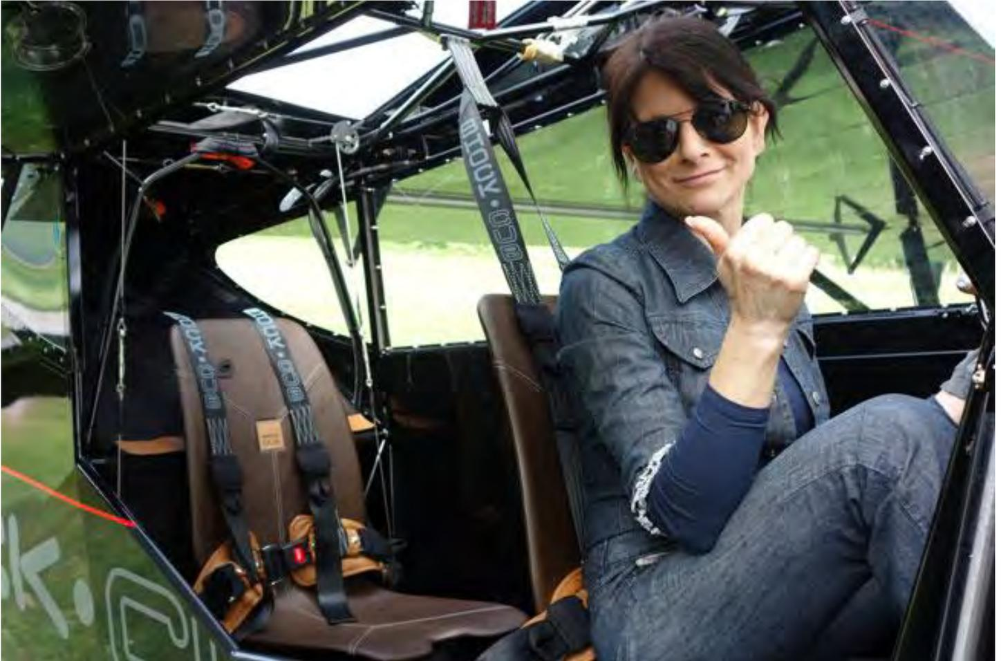
*The spirit of the plane is pure adventure done intelligently. A super-beefy welded chromoly occupant cage, serious restraints and ample escape avenues are the result of safety-first design.*
