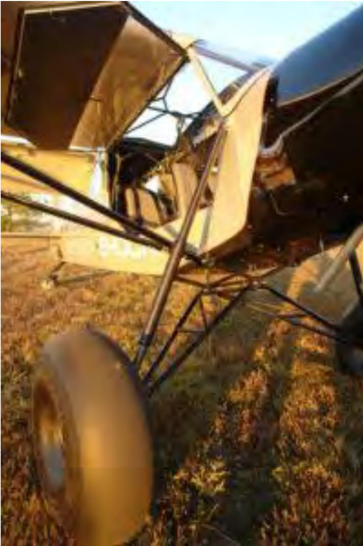
*Absorption much? Let us count the ways: Big tires, giant struts, welded truss-style gear legs and, in back, a shock-absorbing tailwheel, too.*
