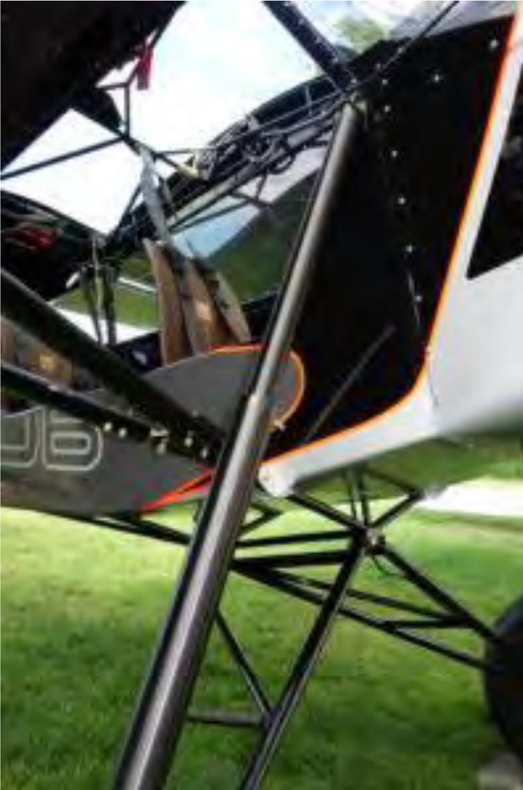
*The cockpit configuration is very much like an old Cub or Super Cub, with the horizontally folding barndoor-style entry. You do solo this bird from the front, like the PA-18 but unlike the J-3.*
