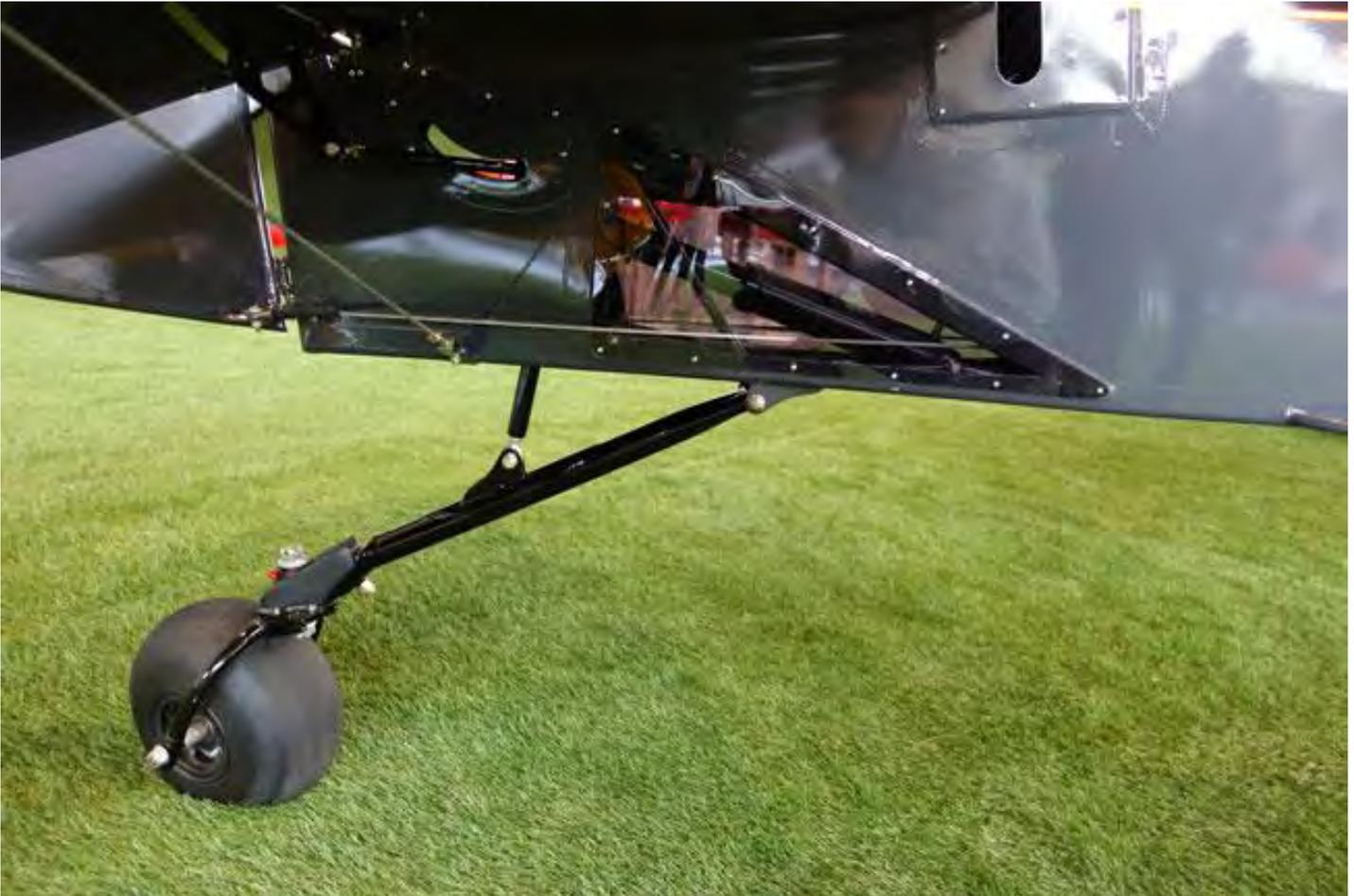
*Shock absorption is important when you're bouncing off near-boulder-sized rocks, so even the tailwheel gets a strut.*
