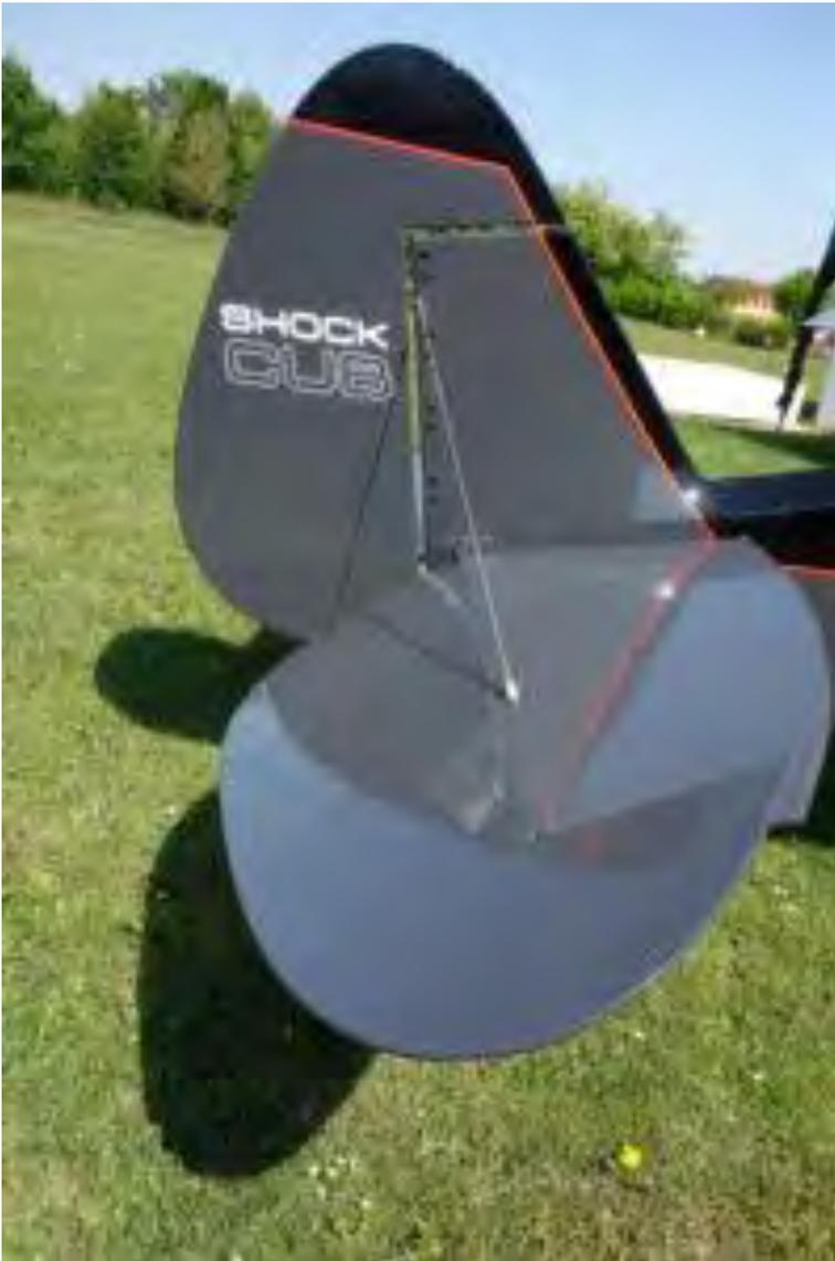
*While it sports a familiar Cub-style shape, the control surfaces are big enough to affect the desired control force even at very slow airspeeds, when air flow slows over the surfaces, too, and might otherwise limit control effectiveness.*
