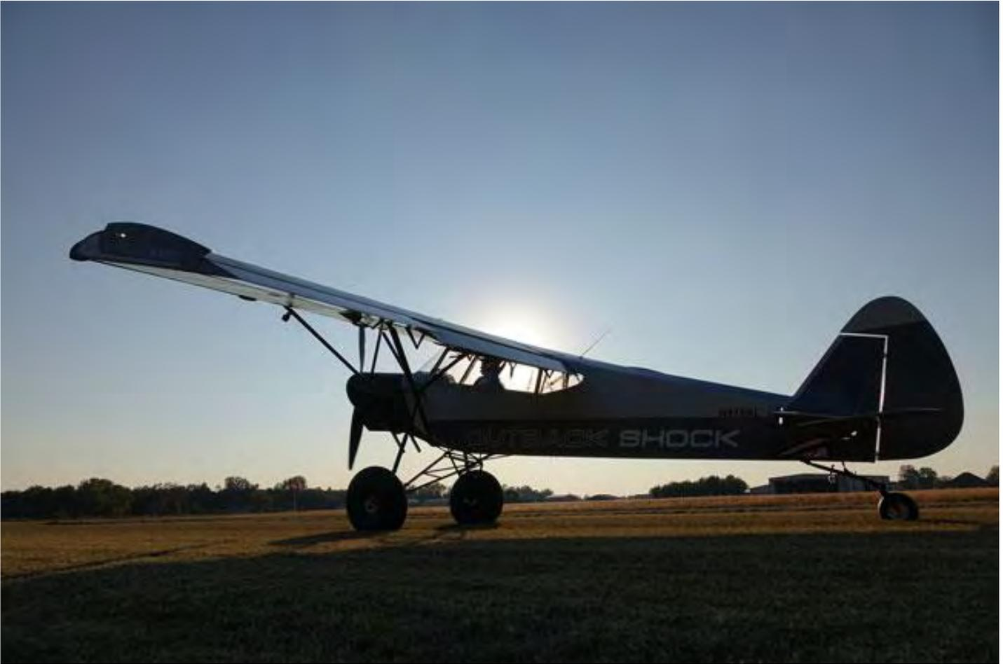
*The Outback Shock needs little more than a small field to get airborne or to set back down again. With its big tires and beefy, shock-absorbing gear, it's rough and ready, and its super-slow landing speeds sweeten the deal.*
